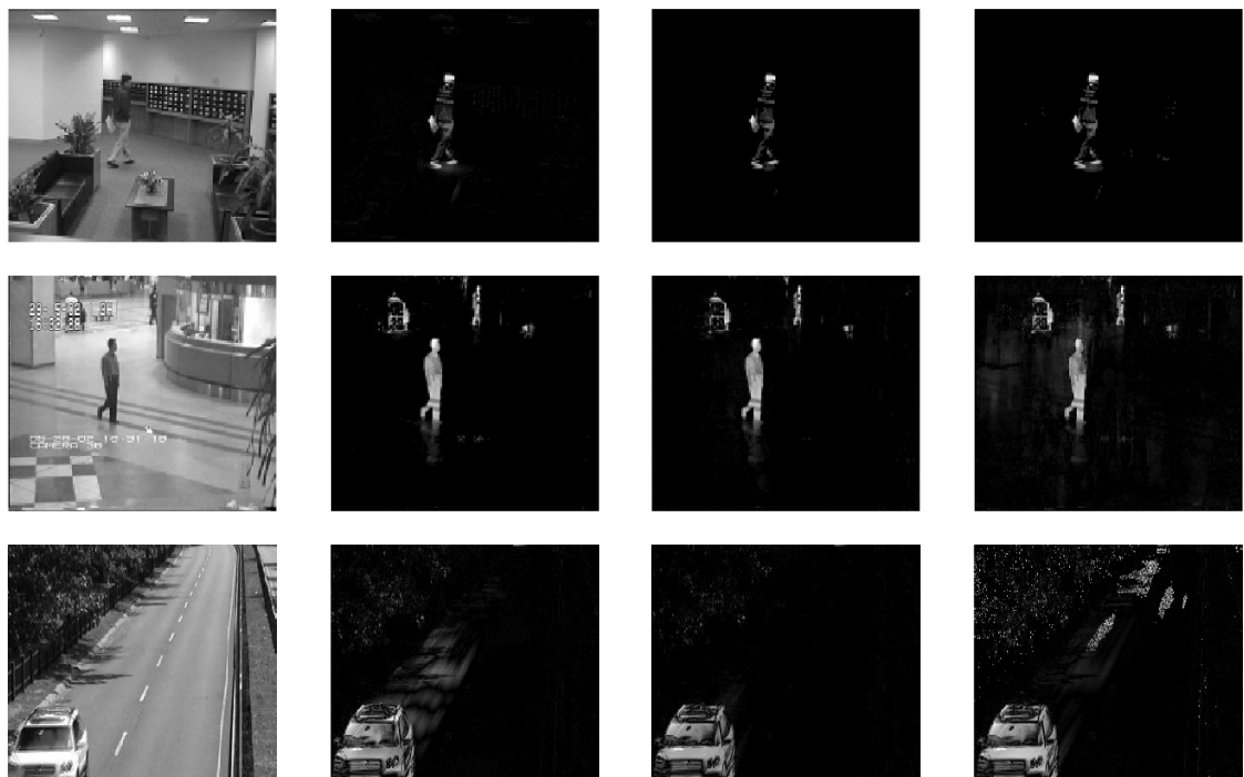
Figure 7.19: Background and foreground separation. From bottom to top row: Highway, Hall, and Lobby. From left to right column: Original video frame, PETRELS-ADMM, GRASTA, and ROBOT.
